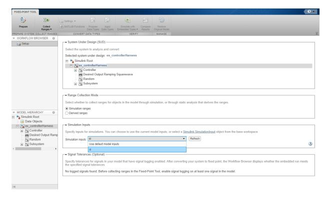
The tool proposes data types based on the merged ranges collected from all simulation scenarios.
