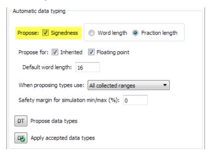
The Fixed-Point Tool bases its signedness proposals on collected range information and block constraints. Signals that are always strictly positive now get an unsigned data type proposal, gaining an additional bit of precision compared to previous releases.
