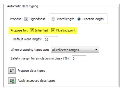
By default, the **Inherited** and **Floating point** check boxes are selected. If you clear the **Inherited** or **Floating point** check boxes, the Fixed-Point Tool will not propose a fixed-point data type for results that use an inherited or floating-point data type respectively.
