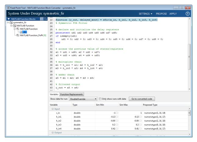
Once you are satisfied with the proposed data types, click **Apply** to have the tool automatically generate a variant subsystem. The variant subsystem contains the original floating-point version of the MATLAB function block, and a fixed-point version of the block. You can refine the conversion by modifying the original floating-point MATLAB code. The fixed-point variant will automatically update after reconverting the block.
